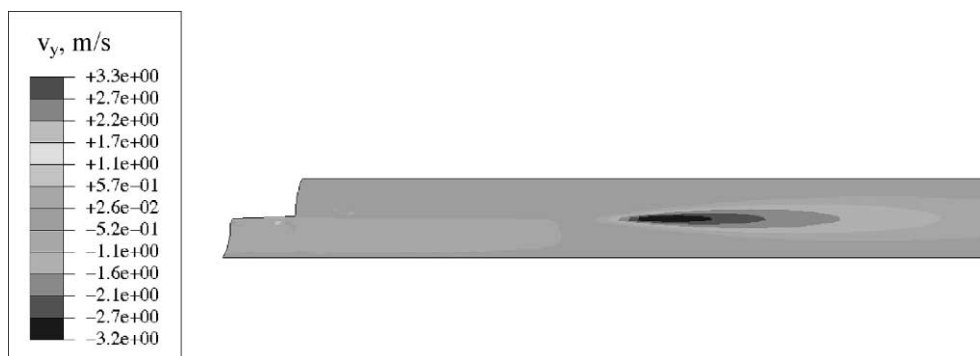
Fig. 4. View of the velocity component v_y at the tip of the shear band for a nominal strain rate of 4 \times 10^4 \text{ s}^{-1} . The negative values of v_y indicate a flow of material from the upper part of the specimen to the lower part.
